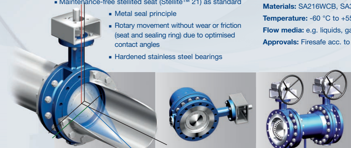
The triple offset design of the process valve guarantees a frictionless rotary movement as well as permanent tightness due to the metal seal principle.
