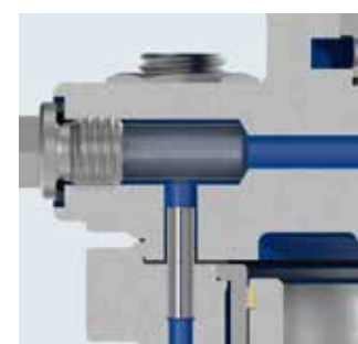
Safer due to additional integrated strainer
